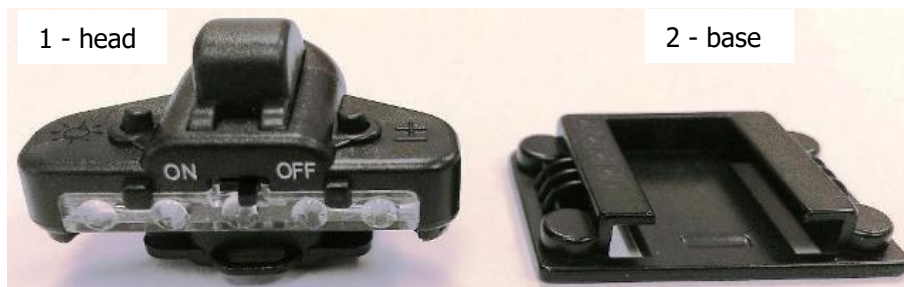
Figure 9: Picture of the AXsys™ Electronic Head part and base part separated
