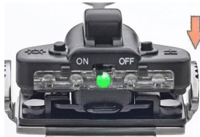
Figure 10: AE-2939 AXsys™ Electronic Toric Head: Sensitivity button location
