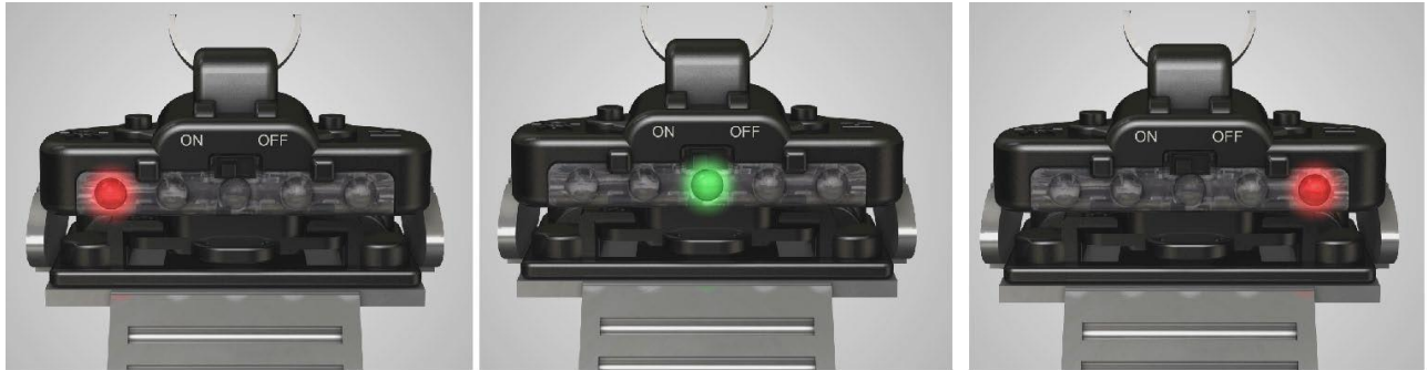
Figure 13: Indications of the brightness level setting in the Electronic Toric head
