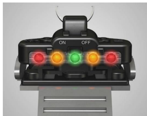
Figure 15: After a successful reset, the five LED lights sequentially illuminate until device is tilted to horizontal.
